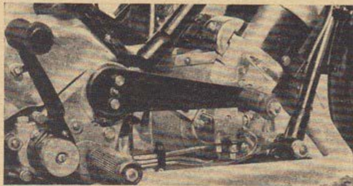
The positive-stop, foot-change operation of the Scott gearbox.
