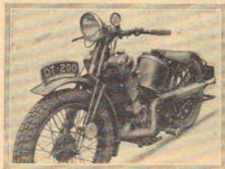
The machine completed. The exhaust from the "Paramount" detachable-head cylinder block is led through the modified front down tubes
